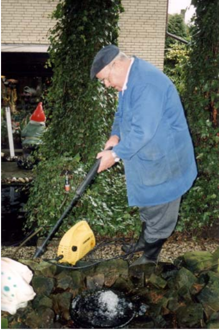
Using a small high-pressure cleaner for cleaning requires a pipe separator for the water connection - only a few house owners know about it (Figure: J. Scheele)
