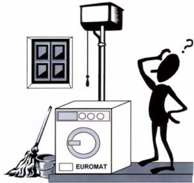
European washing machine connection? Washing machines or dishwashers that are not intrinsically safe must actually be connected via a free outlet (Figure: J. Scheele)
